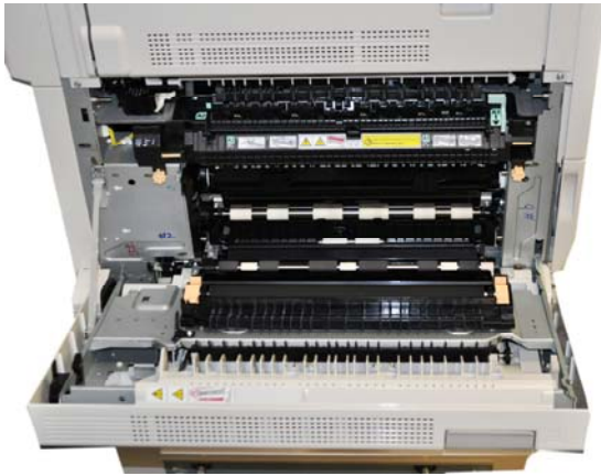
Above: To access the left side misfeed areas, the user first opens the side door. Once open, the user can use the orange levers to open areas to clear any misfeeds.
