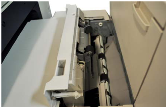
Above and below: When the Office Finisher is attached, users can clear misfeeds on the top paper transport path by lifting the panel up. Misfeed can also be cleared in the front by opening the finisher door and following the directions on the control panel or the door.
