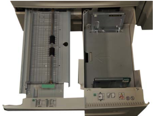
Above: The 2,000-sheet High Capacity Tandem Tray can hold A4 paper and can be loaded while in operation, decreasing downtime.
