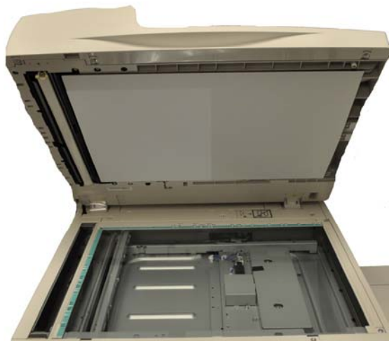
Above and below: The Xerox WorkCentre 7120T platen glass and duplex automatic document feeder (DADF).
