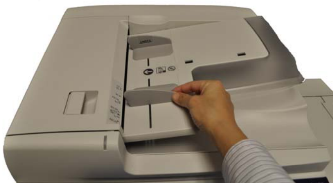
Above and below: The Xerox WorkCentre 7120T platen glass and duplex automatic document feeder (DADF).
